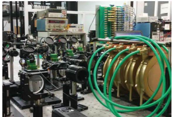
LInC personnel are developing technology for combining multiple fiber lasers into a single high energy beam for application to high energy laser weapons.
