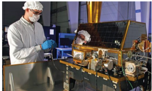
The LInC's Commercially-Hosted IR Payload (CHIRP) is the first military-wide field of view, staring array sensor launched as a hosted payload on a geosynchronous COMSAT.
